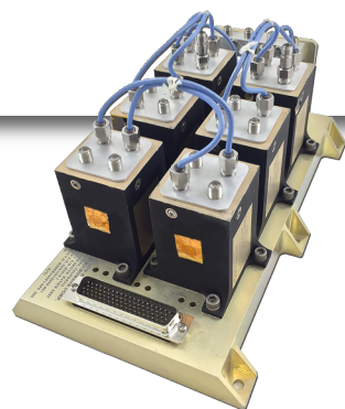
H9010 Switch Block, 6x C Switches, 2x Power Dividers
