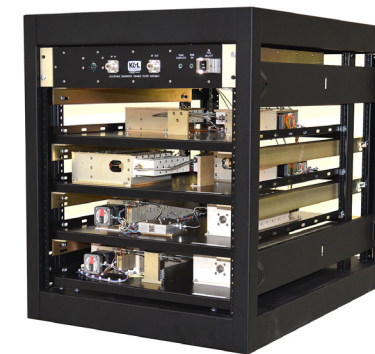
Digitally Controlled Tunable Rack Assemblies • Bandpass and Bandstop Options • Tunable Center Frequency • Tunable Bandwidth • Tune over Multi-octave Ranges • Suitable for LTE and WiFi Testing
